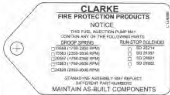
The above tag is stamped to identify the “As Built” Components. Refer to the next two tables to identify:
