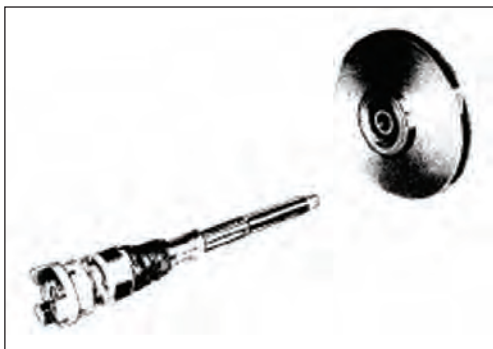
F. Impeller removed from outboard rotating element.
