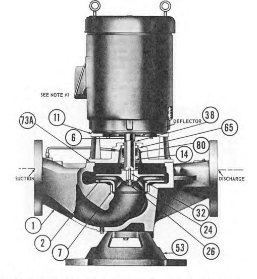
NOTE 1. Conduit box located 45° clockwise from suction flange as viewed from motor end (motor may be rotated in 90° increments).
