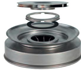
Internal leakage caused by pressure differentials within the pump was minimized. Tests have shown that an impeller seal clearance gap of just 0.016" between the impeller and the chamber causes a 5% drop in efficiency. When liquid seeps out into the pump, precious energy is wasted on circulating that liquid. Grundfos uses a floating seal ring between chambers, providing a nearly perfect seal.
