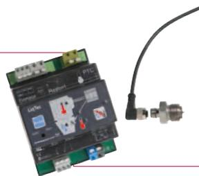
In the event of dry running, the Grundfos LiqTec™ immediately shuts down the pump before damage occurs
