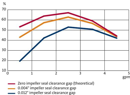
Grundfos achieved a 10% increase in pump efficiency through three innovative improvements to the impeller and seal. These improvements also mean a smaller motor can often be used to power the pump—and that equals savings on both initial investment and running costs.
