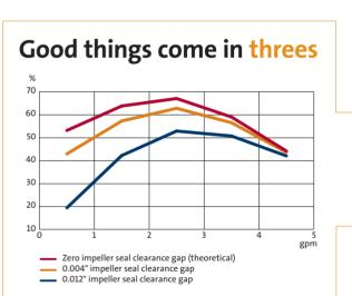
Grundfos achieved a 10% increase in pump efficiency through three innovative improvements to the impeller and seal. These improvements also mean a smaller motor can often be used to power the pump—and that equals savings on both initial investment and running costs.
