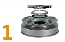
Internal leakage caused by pressure differentials within the pump was minimized. Tests have shown that an impeller seal clearance gap of just 0.016" between the impeller and the chamber causes a 5% drop in efficiency. When liquid seeps out into the pump, precious energy is wasted on circulating that liquid. Grundfos uses a floating seal ring between chambers, providing a nearly perfect seal.
